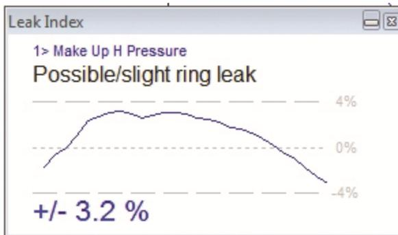
The final example has a line that is rounded, which is an indication of a ring leak. The mass quantity of gas is first increasing, but as the differential pressure changes between head-end and crank-end, the Leak Index curve begins to go down.
