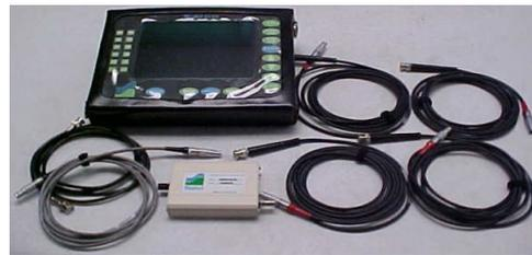
If a Bently Nevada™ panel is installed on the unit, the Prox Trigger can be used instead of an encoder for a TDC pulse by using a BNC-to-BNC cable. Attach the Bently Nevada™ key shaft phaser output to the trigger module. A BNC-to-lemo voltage prox interface cable is needed for each proximeter on which you want to take simultaneous measurements. Keep in mind that the sensor point setup needs to be correct. Bently systems often use a 100mv per mil sensor instead of the 200mv per mil sensor.
