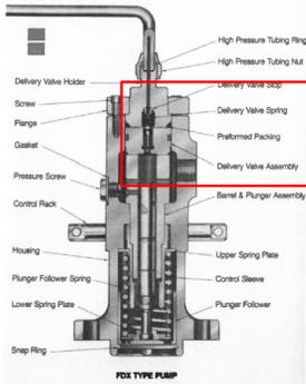
(Figure 4) Fuel Pump Assembly.
