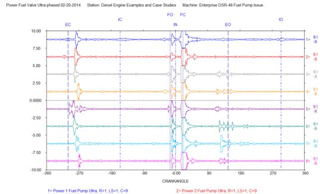
(Figure 7) Normal Ultrasonic data.
