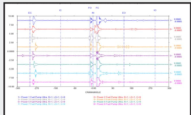
(Figure 1) Initial dataset showing low pressure on cylinder 2. (Figure 2) ultrasonic signature on fuel pump indicating the double hit on closure.
