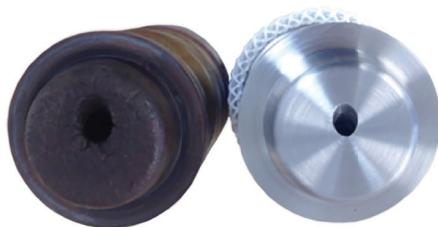
Figure 2 - Old and new pre-combustion chamber ports
