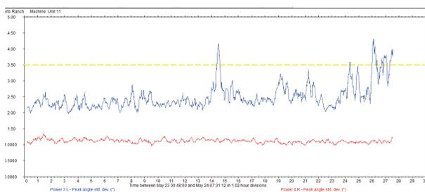
Figure 1 - Standard Deviation of peak firing pressure angle
