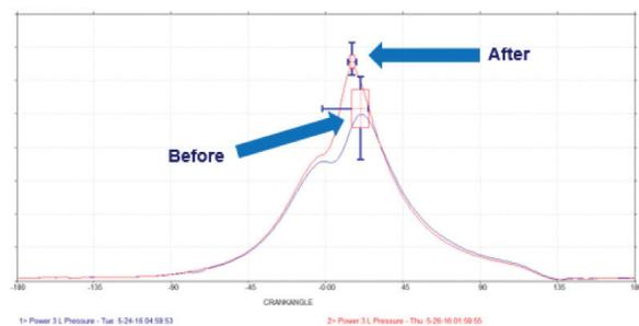
Figure 3 - Before and after power pressure curves
