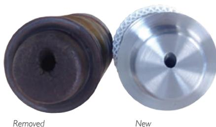
Figure 2 - Old and new pre-combustion chamber ports
