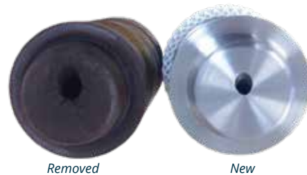
Figure 2 - Old and new pre-combustion chamber ports
